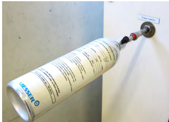
Propane injection for Shed chamber calibration
