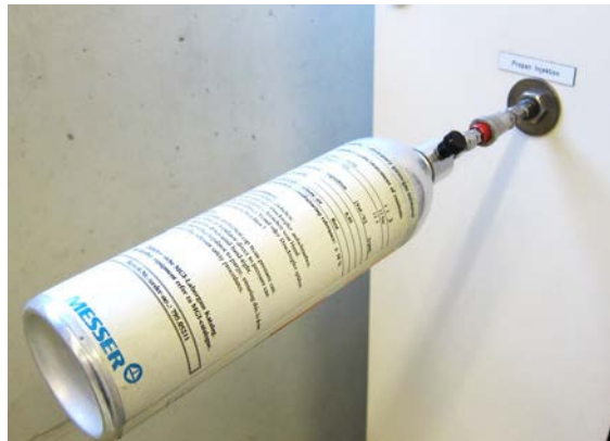
Propane injection for Shed chamber calibration
